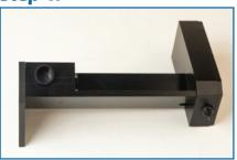
Make sure the cell is always clean and dry. Use compressed air and acetone for this process. Fill the cell from the lower inlet port with a Luer Syringe only. As the cell becomes filled and sample begins to appear at the upper inlet, cap off the upper then lower inlet port. Your cell is now filled and air bubble free.
